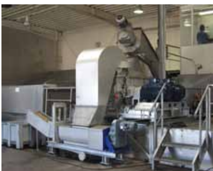
SEPARATING AND CRUSHING OF PACKAGED FOOD WASTE AT SEVERAL LOCATIONS FOR A LEADING RECYCLING COMPANY.
