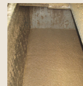
After separation in the mill, the organics (liquid phase) are pumped into a storage tank for further processing.
