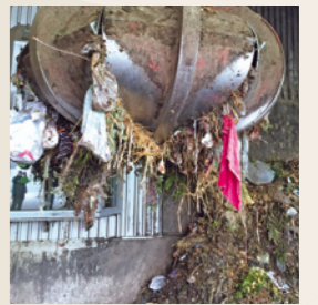
The input material is conveyed into the DRM grinding chamber via a receiving container and a screw conveyor.
