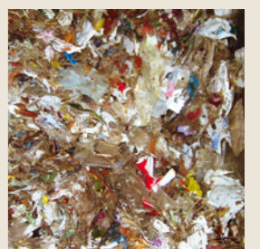
The foreign matter and impurities (solid phase) drop from the mill directly into a press screw.
